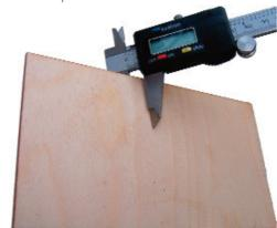
The original design was made to fit .124" thickness materials. If we select everything in the design and proportionally change the size it will go together perfectly. Let me show you what I mean. The new plywood I just bought measures out at .133" thick, so I
